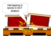
Figure 4 Overlapping of wire spools
